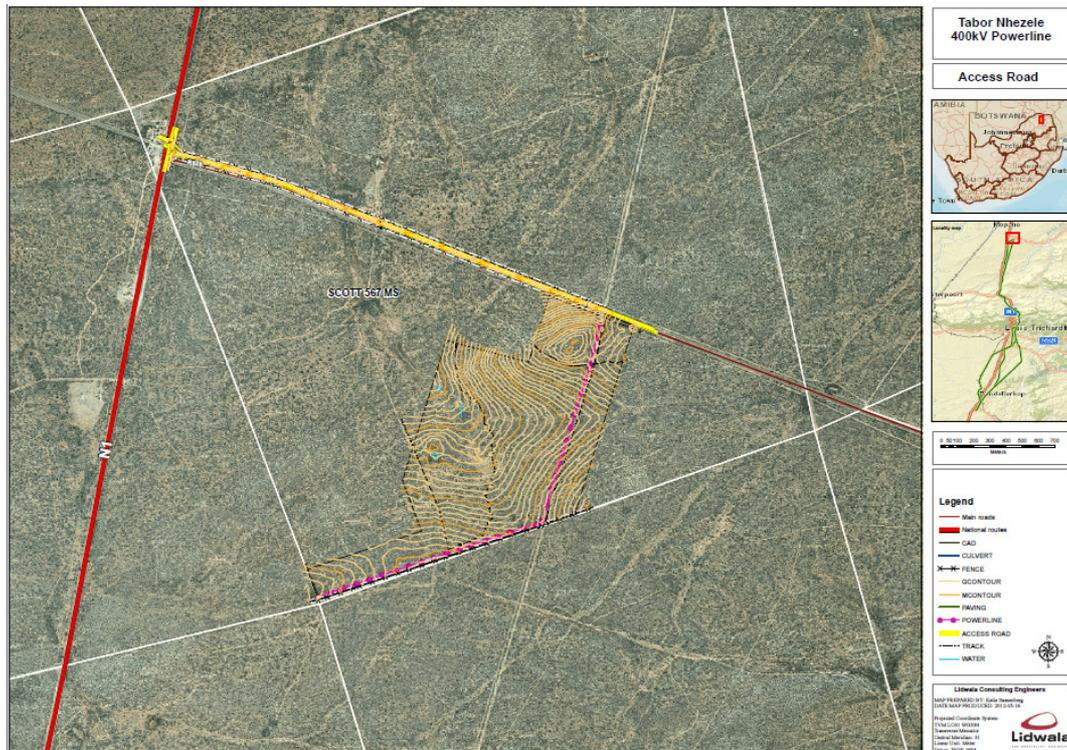
**Figure 10.4:** Proposed formal access road to the proposed new Nzhelele substation
